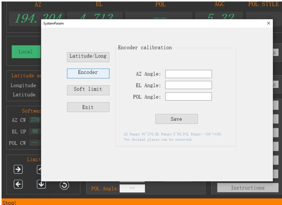
Figure 4-21 Encoder Calibration
