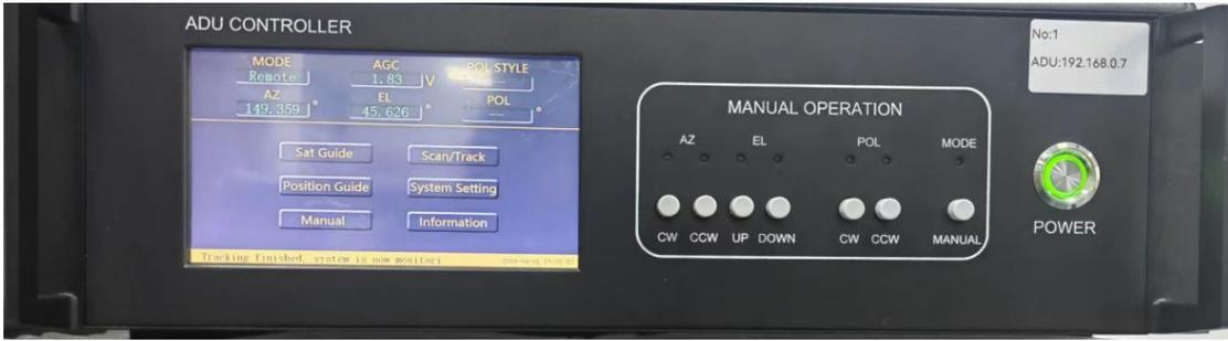
Figure 4-7 Manual Control Panel of ADU Controller
