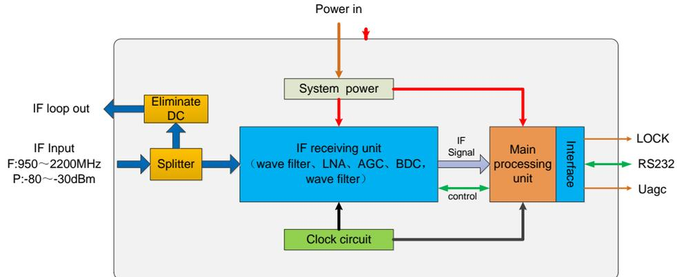
Figure 3-6 Schematic diagram of beacon receiver
