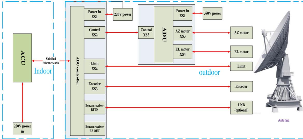
Figure 3-1 System Diagram
