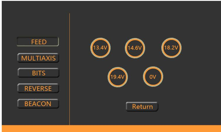
Figure 5-1 LNB Feed Setting
