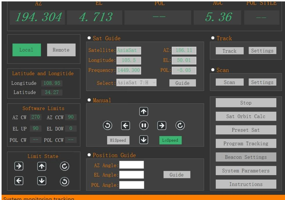
Figure 4-12 Remote Control Interface
